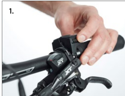
Switch the battery on using the on/off button on the system. The screen takes a few seconds to display the start screen.
