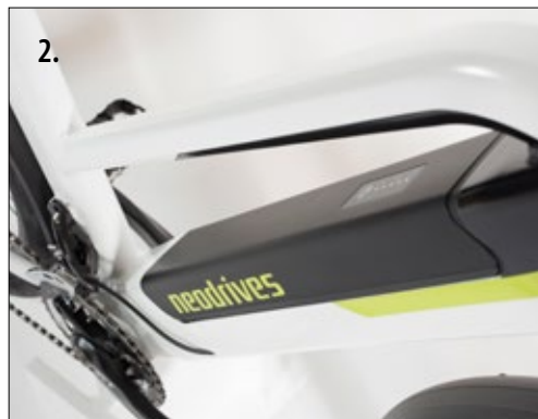
Semi-integrated battery with battery button: no need to press the battery button.
