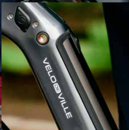
Battery integrated into the frame for a cleaner look and more capacity
