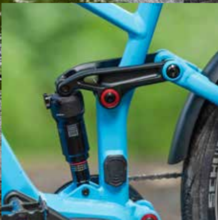
Unique comfort thanks to the suspended frame
